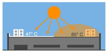
On a clear day, roof surfaces are exposed to direct sun radiation. A heat pocket is formed above the roof surface with air temperatures significantly above the surrounding environment.
