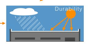
Buildings with ZEFFLE IR - coating on one hand achieve a passive cooling effect which reduces the cooling load. On the other hand ZEFFLE IR lowers the ambient air temperature, which reduces the power consumption of heat pumps in cooling mode.
